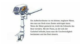
An outboard motor is a small, portable motor which can be attached to the stern of a boat. When the motor is started, the propeller moves the boat forwards. The tiller, which also has the throttle on it, controls both the direction and the speed of the boat.
